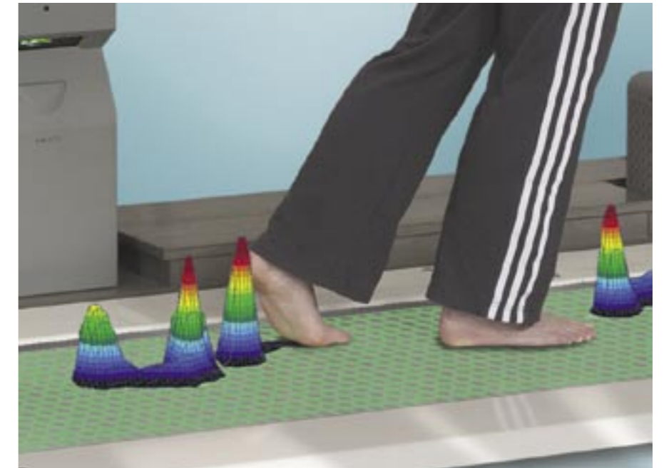
The sensor plate contains a matrix with calibrated capacitive pressure sensors that can be perfectly be integrated between parallel bars. The evaluation is produced on a PC.
