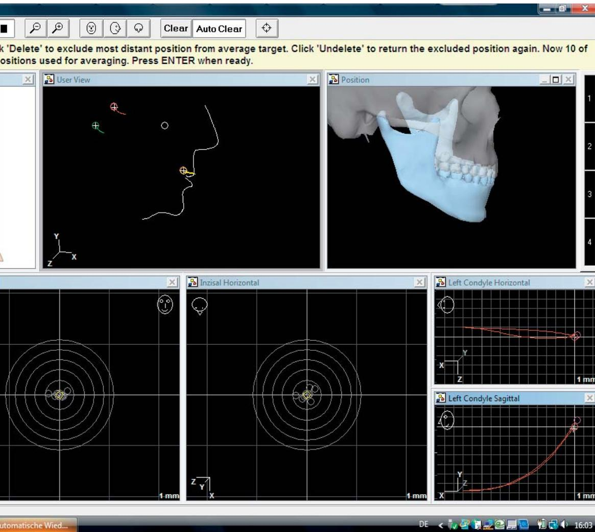
On the measuring screen for determining the neuromuscular jaw relation, the position of the incisal point is shown together with the condyle positions. Once the optimum jaw position has been determined, it can be compared for checking purposes with the retruded, habitual position. The incisal point can be superimposed with arrow angular movements.
