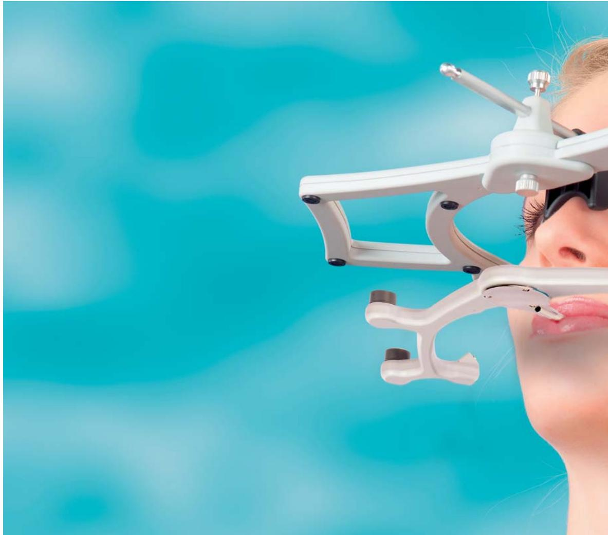
The zebris Jaw Measurement Analysis System records all the 3D movements of the lower jaw without contact, using the principle based on measuring the travel time of ultrasound impulses. This system consists of a face bow with integrated receiver sensors and a lower jaw sensor for measuring near the joint, that is optimally balanced. The reference plane, e.g. the axial-orbital plane, is entered using a probe
