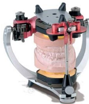
For programming fully adjustable articulators, tables for the settings and measuring curves are shown clearly in the report. The transfer to the articulators Protar, SAM, ARTEX, Reference, Panadent™ and STRATOS is carried out using commercially available face bows.
