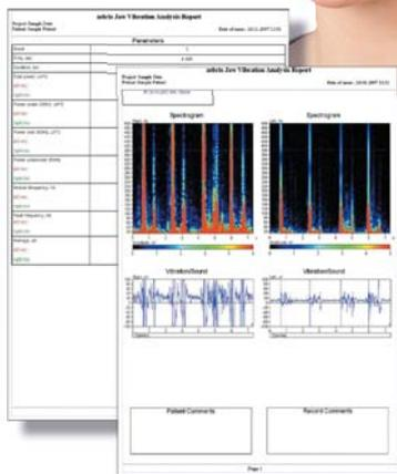
A spectral analysis of the joint noises and a numerical analysis of the cracking sounds is shown in the evaluation report. The movement measurement can be superimposed.
